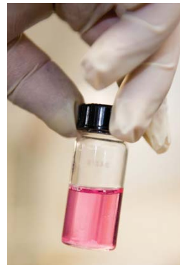
An operator tests a sample of effluent indicating chlorine residual.
